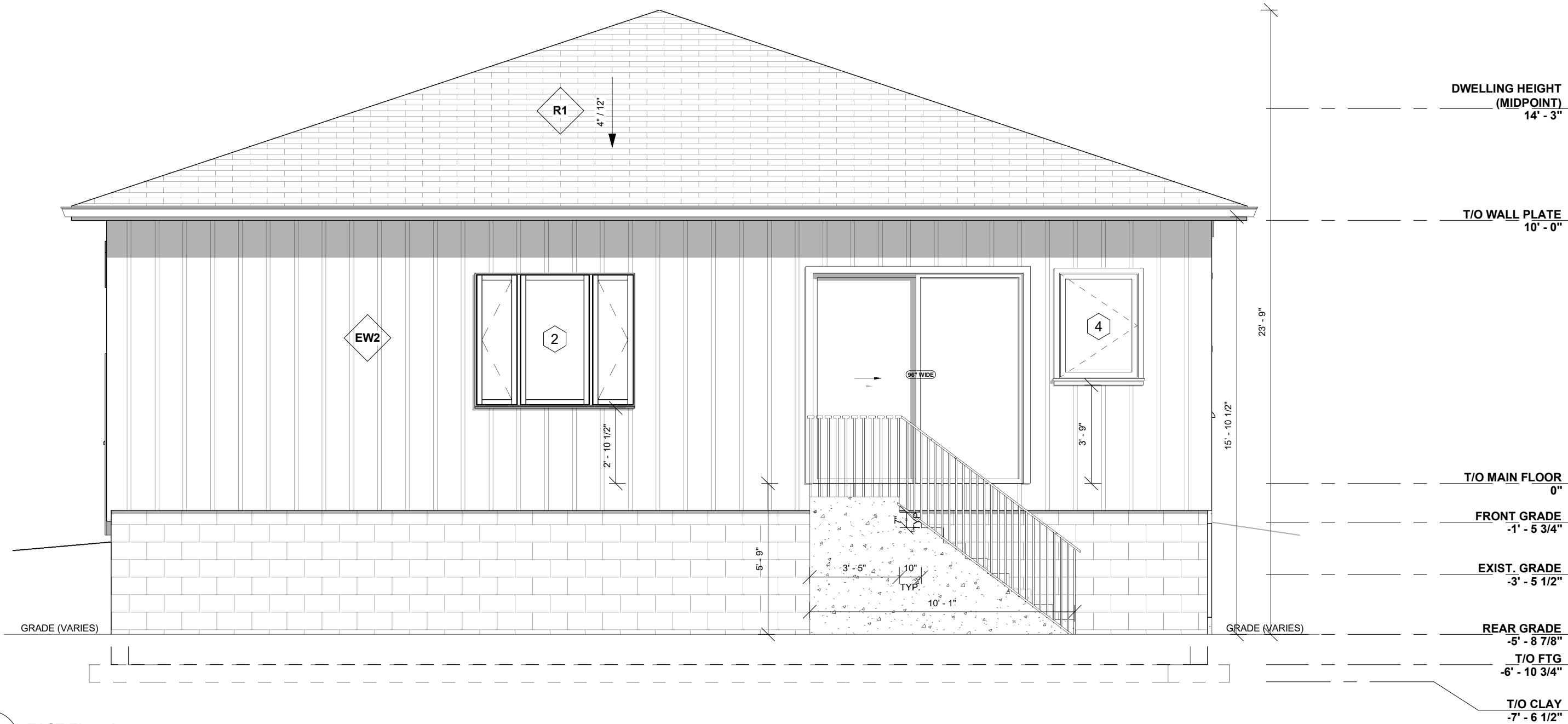
1 EAST Elevation S-9 1/4" = 1'-0"
