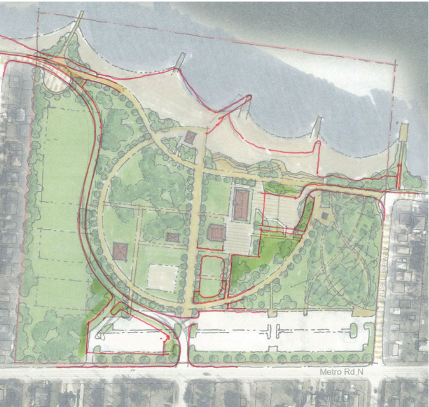
Early thinking on an option to create park/beach uninterrupted by a road by redirecting Lake Drive to Metro Road N on the west side of the park.
