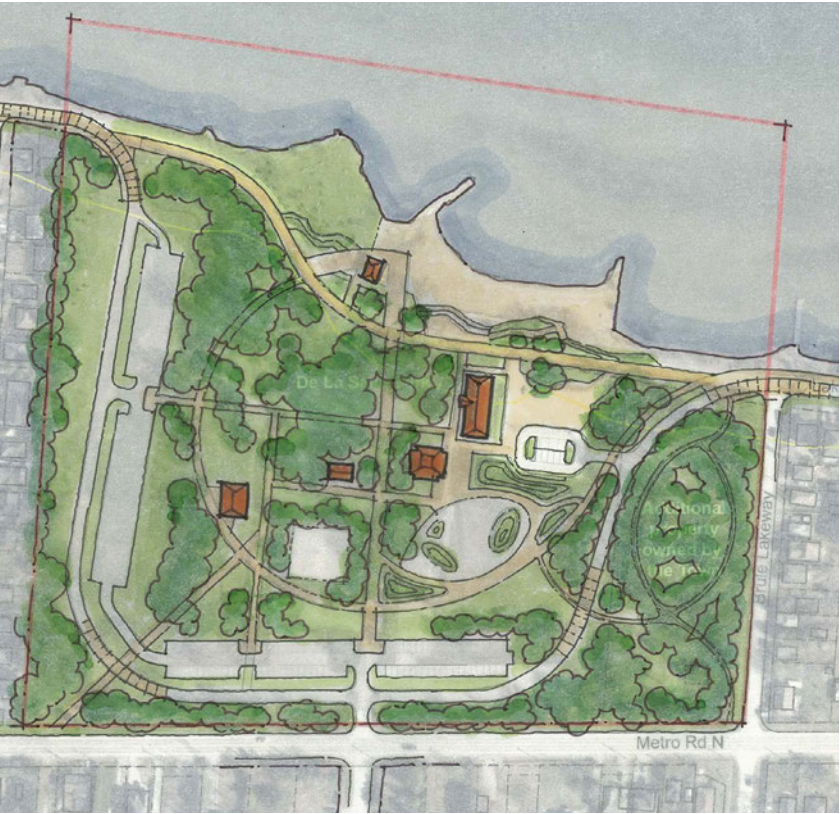
Preliminary concept showing a redirected Lake Drive along the edges of the park to allow uninterrupted connection between the beach and park
