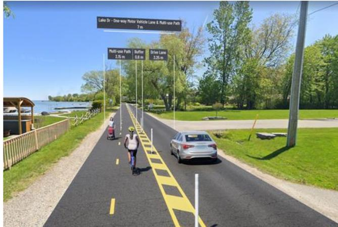
Picture 1: Proposed lane arrangements – Section 2
